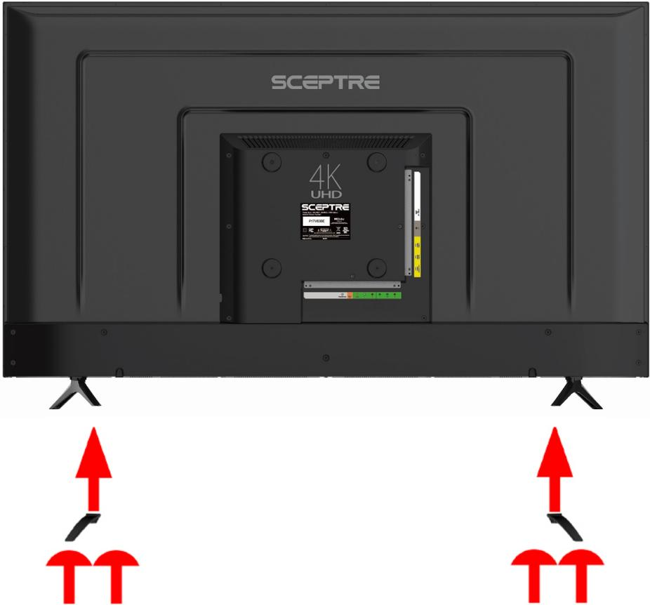
2. Insert and tighten 2 screws from the bottom of each foot.
