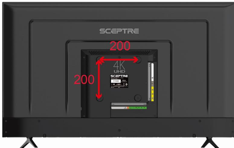
Mounting Specification: **200mm x 200mm** using 4 screws sized at **M6 (not included)**. Length of screw should not exceed **10mm**. Please Note: The **10mm** length of screw refers to how deep the screw can go inside the mounting holes. When you are buying screws, you should add the original 10mm to the thickness of your mounting plate in order to get the total screw length.
