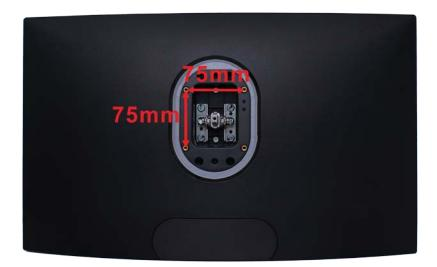
Mounting Specification: **75mm x 75mm** using screw size **M4**. Length of screw should not exceed 8mm. Please Note: The **8mm** length of screw refers to how deep the screw can go inside the mounting holes. When you're buying screws, you should add the original 8mm to the thickness of your mounting plate in order to get the total screw length.
