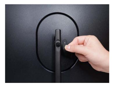
5. Install the display connection plastic cover to the lower part of the display.
