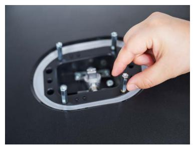
6. Once all 4 spacers are installed the display is ready to be mounted. The mounting specification of the display is **75mm x 75mm using M4 screws at 8mm length**.
