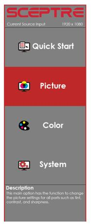
When you press the **M** button on the monitor, the OSD screen will appear. Select each of the functions with the  $\blacktriangle$  or  $\triangledown$  buttons. Use the **M** button again to enter each of the function or when you're in the function already, use the **M** button to select the option you want to adjust. Use the  $\blacktriangle$  or  $\triangledown$  buttons to adjust each option's values. When you want to exit press the **E** button.
