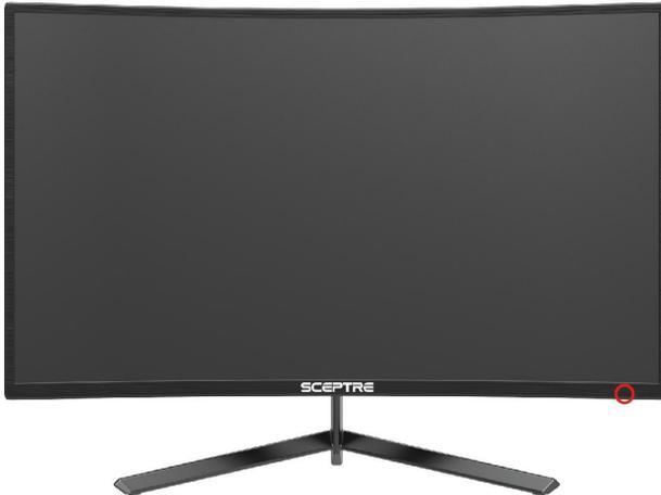
**Indicator Light** – The light is blue when the monitor is turned on. The light is red when the monitor is turned off but plugged into power. The light is flashing blue when there is no signal given to the monitor.
