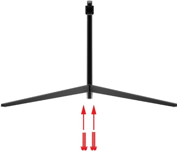
2. Install the assembled stand to the back of the monitor and screw in the 1 neck screws to secure the stand to the monitor.
