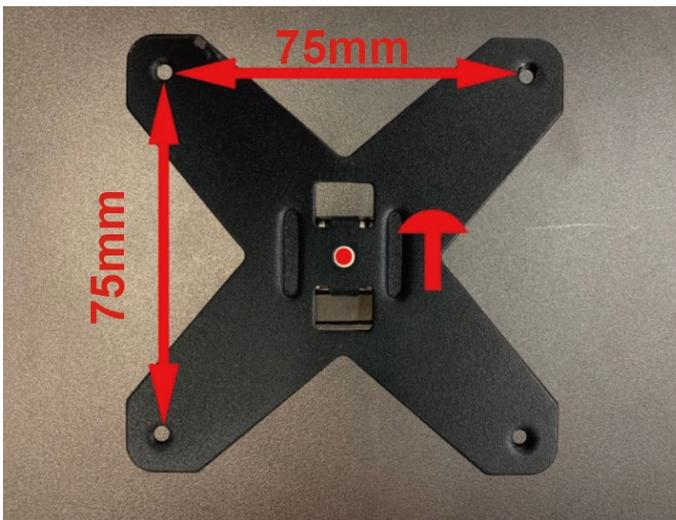
2. Once the stand is removed, you will see the indentation where you can install the mounting plate. **The mounting pattern is 75mm x 75mm using M4 x 10mm screws.**
