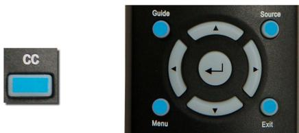
**CC** – Press this button to enable the CC function. You can then use the ▲▼ buttons to select if you want CC off or CC on. You can use the ◀▶ buttons to select between different CC channels.
