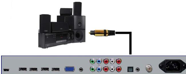
1. Make sure the power of X42 LCD HDTV and your receiver is turned off.
