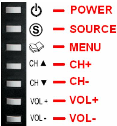
**POWER** – Turn on the TV by pressing the button once. Press the button again to turn off the TV.
