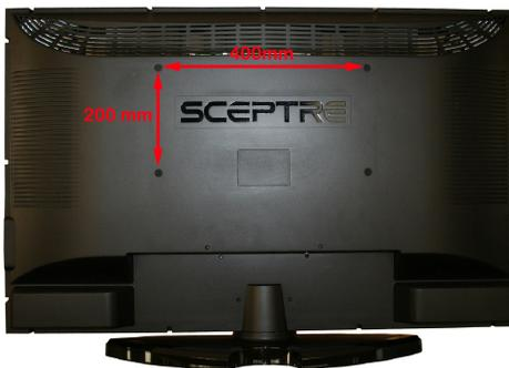
Mounting Specification : **400mm x 200mm** using screw size **M6**. Length of screw should not exceed **12mm**. Please Note : The **12mm** length of screw refers to how deep the screw can go inside the mounting holes. When you're buying screws, you should add the original 25mm to the thickness of your mounting plate in order to get the total screw length.
