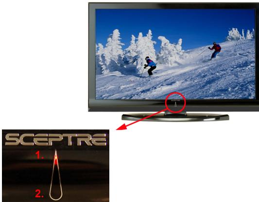
**1. INDICATOR LIGHT** – The light is red when power is plugged in but the TV is not turned on. The light turns blue when the TV is turned on. **Because of the size of the panel, the X42 LCD TV will take 10 – 12 seconds to power on.**
