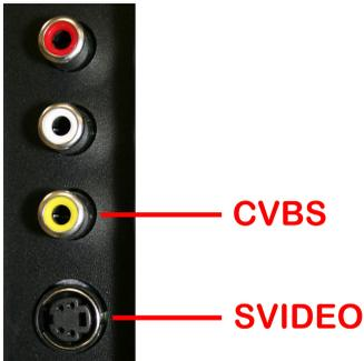
**AV (CVBS)** – CVBS connects to devices that use composite video cables such as VCR or camcorder or video game consoles. Please connect the video portion with the yellow connector. Do NOT connect both yellow and black video connectors. AV shares the audio red & white connectors with SVIDEO.
