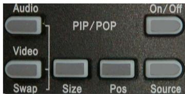
**ON/OFF** – To turn on the PIP or POP, press the ON/OFF button. When you press the ON/OFF button once, PIP will turn on, press the ON/OFF button again and PIP will turn into POP.
