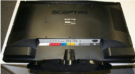
2. Take a look at the neck that's connecting the base to the TV. There should be 4 screws on the neck and 2 screws on the side. Remove the 6 screws and the base will slide off.
