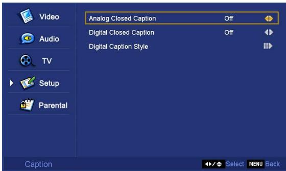
I. ANALOG CLOSED CAPTION – This function cycles through different analog closed caption methods. U.S. usually uses CC1.
