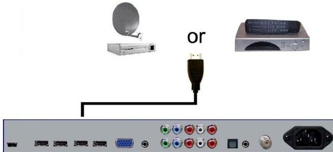
1. Make sure the power of X42 LCD HDTV and your set-top box is turned off.
