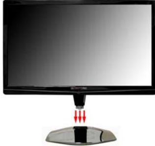
2. Similarly, to remove the stand for wall mounting, simply remove the 4 screws at the bottom section of the TV and pull out the stand. **The 4 screws in the package are for securing the monitor stand only. If you are mounting the LCD, please consult a qualified installer for further instructions on bracket support and wall support.**
