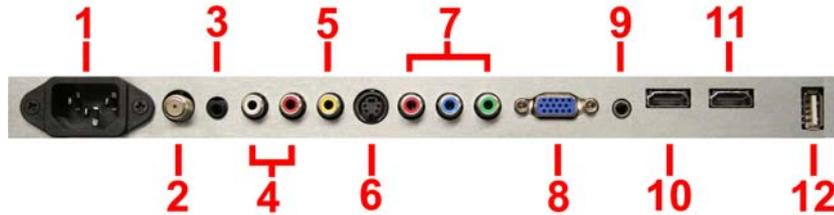
1. **AC** – This connection is for providing electricity to the TV.
