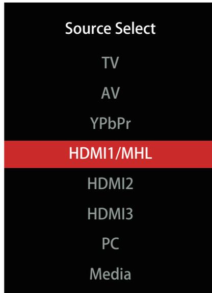
1. Press the **S** button on the side of the HD Display or the SOURCE button on the remote control and you will see the picture above.
